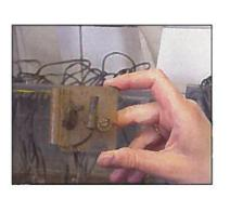
This monitor uses a reed switch to detect whether the mussel's shell is open or closed. The mussels close their shells when sensitized by a toxicant.
